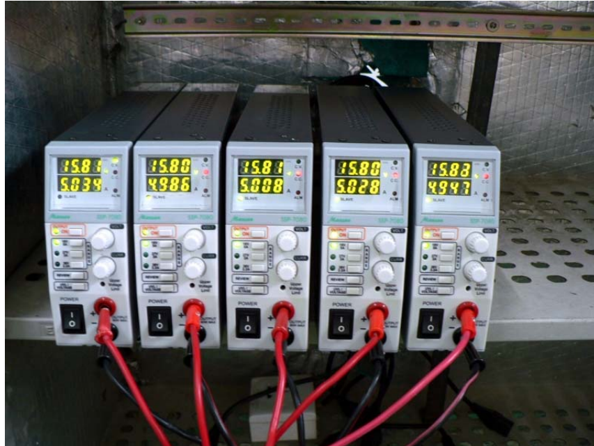
Figure 1 Front panel of Multi-VI range, scalable power supply SSP-7080 in action. All units have been set with the same VI range (16V, 5A)as shown on the indicators.
