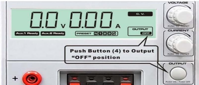
2. Press and hold the voltage knob for about 5 seconds to enter into the setting mode with flashing “Preset Icon” as shown below.
