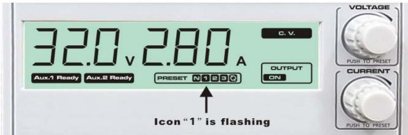
2. Adjust Voltage Knob for voltage value and Current Knob for current value.
